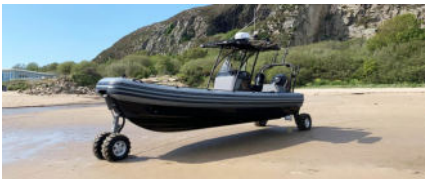
fishing boat with powered wheels!
